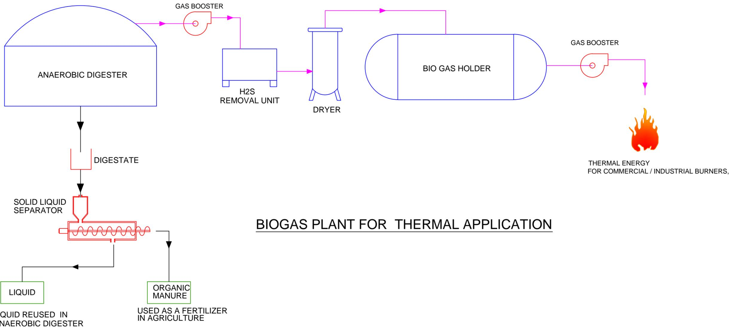
**BIOGAS PLANT FOR THERMAL APPLICATION**
